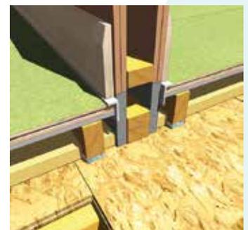
Internal Wall Junction Loadbearing (Rip Liner alternative detail)
